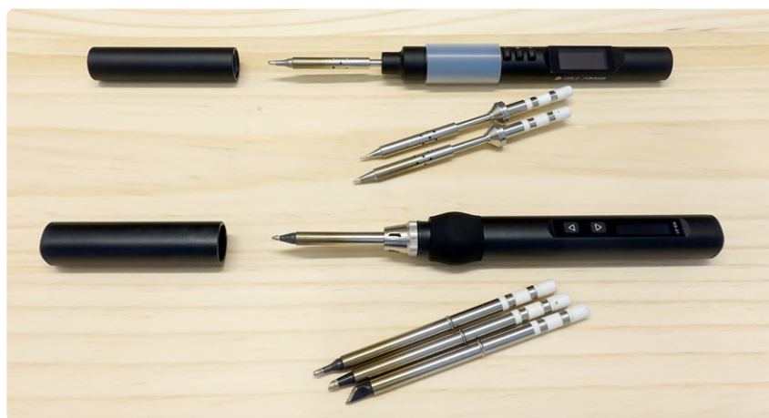
Figure 6: Two portable soldering irons, ideal as secondary irons. Check particular models as cartridges are not always interchangeable.
