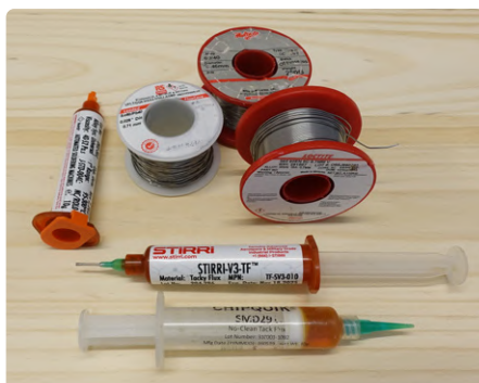
Figure 8: A selection of solder wires and flux.
