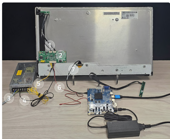
Example Setup, Back: (1) Backlight Cable, (2) LED Backlight Driving Board, (3) Schuko Power Cord, (4)(5) Power Supply for Backlight Driver, (6) Backlight Control Cable, (7) Signal Cable.
