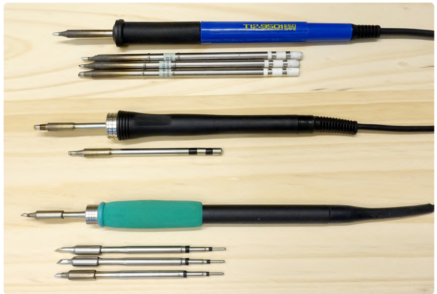
Figure 2: A selection of cartridge systems: Hakko T12, Elektor/Atetool AE970D, JBC C245.
