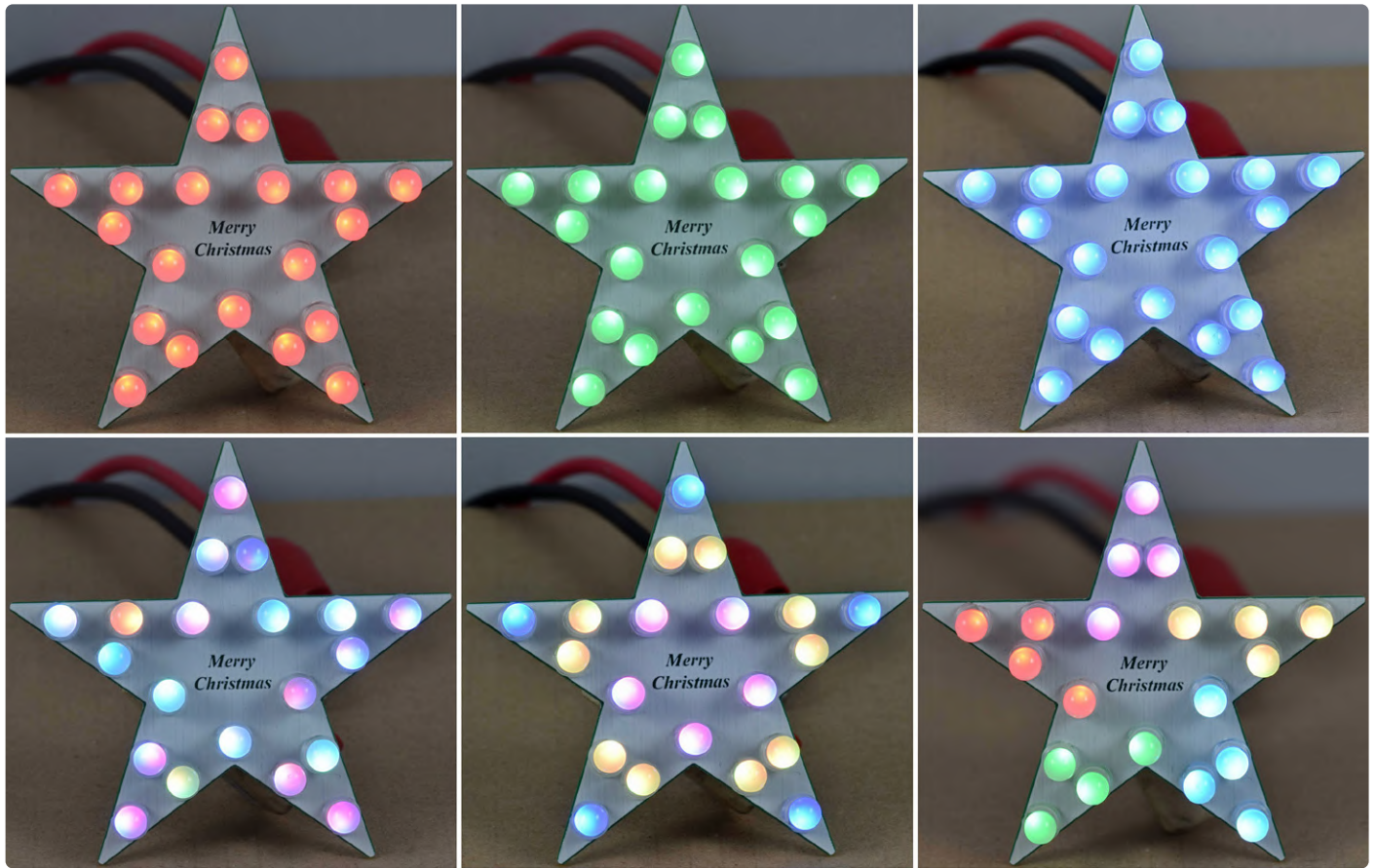
Figure 8: Photos of different patterns to give a first impression. In reality the LEDs appear much more brilliant. Upper row from left to right: All LEDs are red, green or blue. Lower row from left to right: Random changing colors, seven colors shift outwards and colors rotate clockwise.
