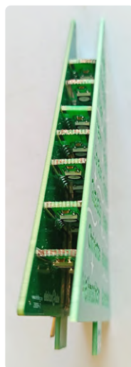
Figure 3: Each word has its own compartment lit by its own LED(s).
