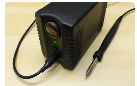
Figure 3: Just an on/off switch and nothing else on this Metcal PS-900: not adjustable, but tons of heating power.
