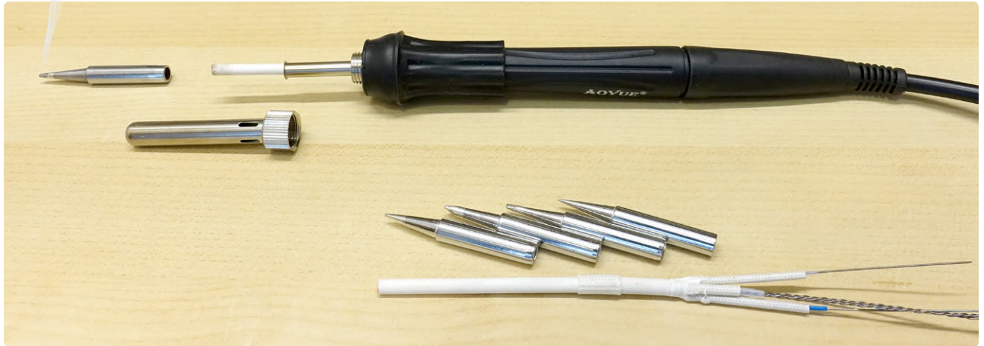
Figure 1: Traditional iron with separate heating element and soldering tip.
