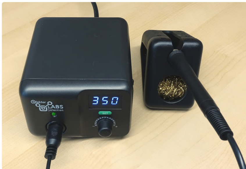
Figure 5: The AE970D, a simple cartridge-based soldering station with an easy to use interface.
