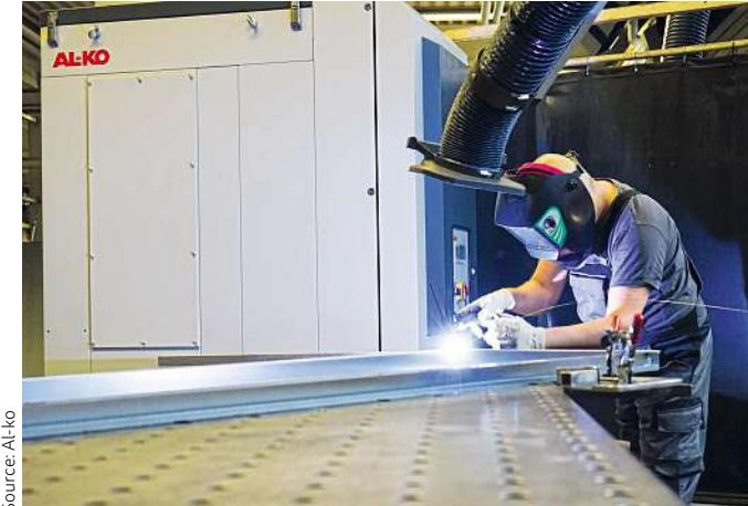
Equipped with extraction arms, the mobile welding fume filters of the Al-ko Clean Unit F series remove fumes even during manual welding.
