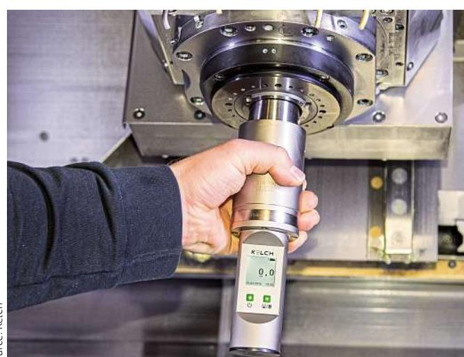
The force gauge covers a measuring range from 2 to 100 kilonewtons.
