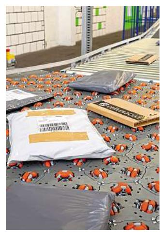
Polybags on a Cellumation conveyor line: even such bags can be conveyed on a large scale in a small space.
