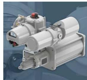
The SI range of actuators from **Rotork** combine the simplicity of electrical operation with the precision of hydraulic control and the reliability of mechanical spring-return fail-safe action. Typical applications for Skilmatic SI actuators include functional safety-related Emergency Shutdown (ESD) inputs
