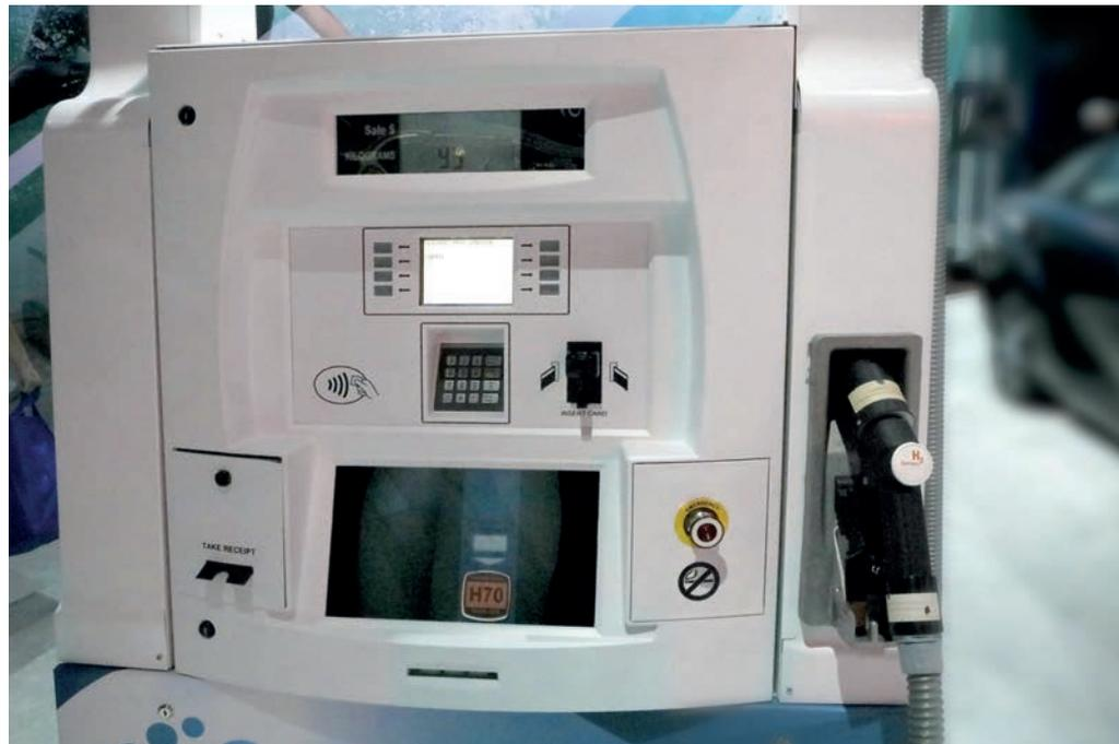
*The measuring solutions in the H<sub>2</sub> refuelling process must work reliably over a long period at pressures of up to 900 bar and temperatures from -40°C to +85°C ©: istockphoto*
