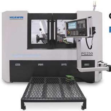
**Gear Profile Grinding**
