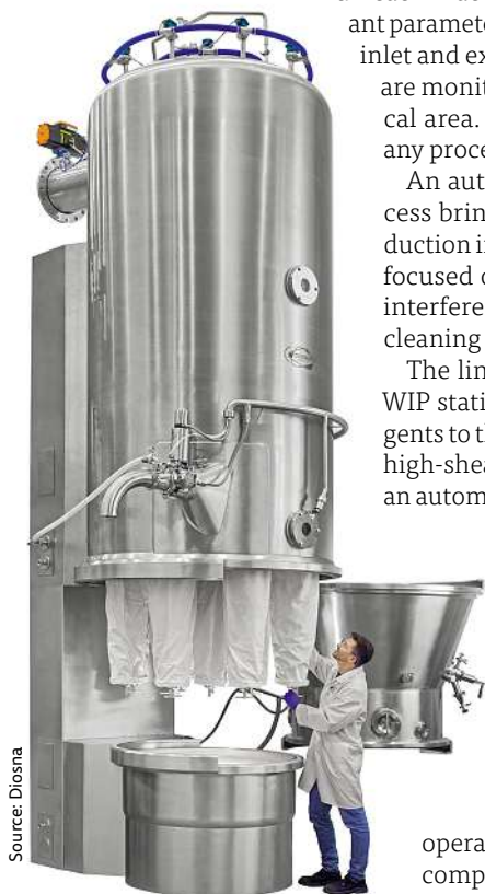
Diosna CAP1250 fluid bed dryer with the filters lowered.
