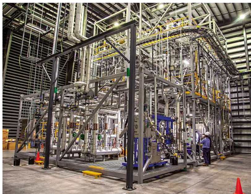
Purecycle Technologies' feedstock evaluation unit: The project involved the advanced processing of recycled polypropylene to convert it to ultra-pure recycled polypropylene.
